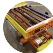
Power-rollers to interface with facility conveyer systems
